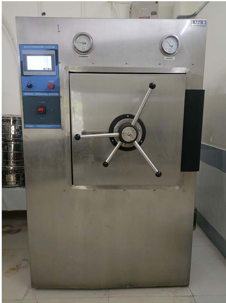
Figure No. 2: Autoclave.
